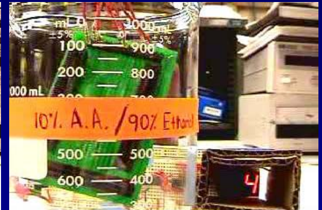
Sensor in Ethanol with 10% -COOH vapor Reading: 4
